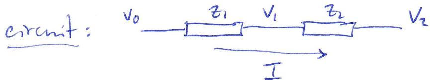
Z's are impedances:  $V_0 - V_1 = Z_1 I$ ,  $V_1 - V_2 = Z_2 I$  (Ohm's law)
